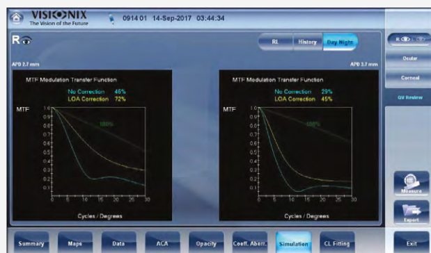
Objective day and night refraction measurements. Analysis of aberrations with Zernike coefficients
